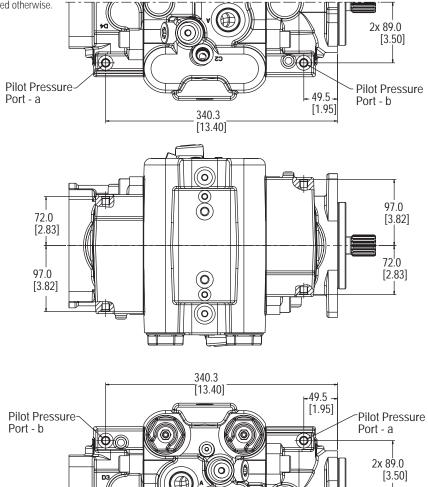
Pilot pressure ports a, b - 0.4375-20UNF-2B SAE O-ring ports
