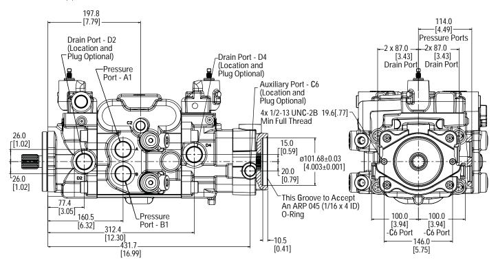
350 Series Dual Pump, Solenoid displacement control, SAE C mounting flange, 14-tooth, 12/24 pitch spline, SAE B Aux mount without charge pump, opposite side ports.
