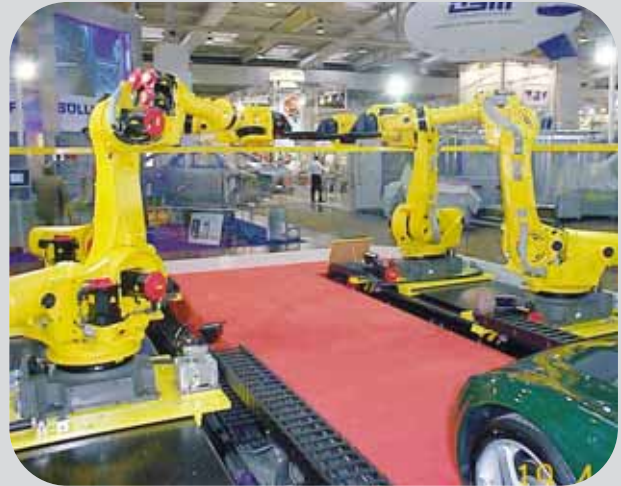
igus® ReadyChain® used for travel axes for 6-axes robots - standard filling with additional options
