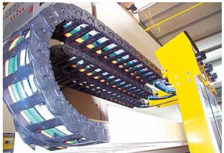
igus® Chainflex® cables also allow for minimum bending radii of 5 \times d together with millions of strokes.
