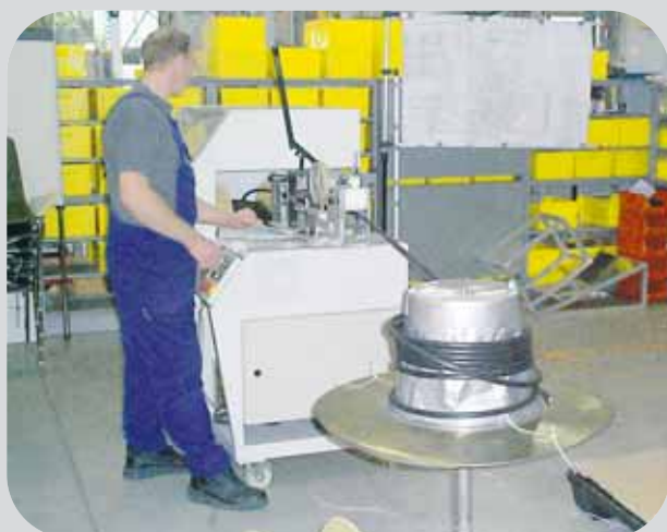
Non-spinning cable handling for more safety
