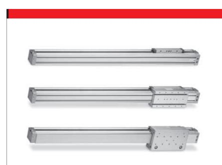
The rodless cylinders Series 52 are available in 5 diameters (25, 32, 40, 50 and 63 mm) and comes in three main versions: Basic (M), with Slide bearing (G) and with Roller bearings (R). Furthermore these three main versions are each available with either standard- or short carriage to cover a wider range of applications.
