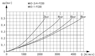
Reference diagram for models with filtering element = 1  $\mu$ m
