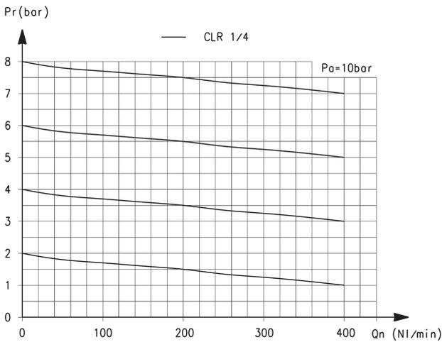
Pa = Inlet pressure - Pr = Regulated pressure
