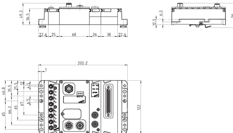
**Digital outputs module with D-SUB - 37 pin connector Mod. ME-xxxx-DD**
