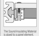
The panel element should be fastened in the profile frame in such a way that as little vibration or sound is transmitted as possible.
