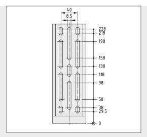
compatible with the modular dimensions of Lines 8, 10 and 12. The slotted holes for fastening to the side face of a profile are
