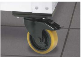
Unlike Castor D125 swivel with double-brake heavy duty, the N version allows the lock to be actuated from the trailing side. The combination of two Castors D125 swivel with double-brake and two Castors D125 swivel with double-brake N thus enables a heavy structure on swivel castors to be locked at all four castors, since the locks can always be reached easily. This prevents the structure from being moved or rolling away.
