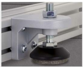
Foot Mounting Bracket 8 D80 allows height adjustable feet with M16 threaded spindle (primarily Knuckle Foot D80, M16) to be mounted on the side of a frame construction. Machines or systems can be installed with minimum distance to the floor but can still be adjusted in height.
