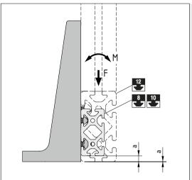
In the case of Line 8 profiles, the distance to the floor when using the lower groove for attaching the L-Based Foot is a=9.5 mm. In the case of Line 10 profiles a=4.5 mm. Line 12 profiles can be screwed to the L-Based Foot so that they are flush to the floor.
