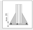
The height can be adjusted by means of a screw inserted into a thread in the core bore in the end face of the stand profile. Floor-Fastening Sets 355
