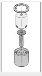
The spindle is screwed into an M8 thread in the core bore of the profile. Tools are not required to make height adjustments – simply turn the lower part of the foot manually.
