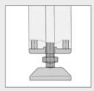
The Foot Cap is clamped in the outer profile cavities of the Profile 8 40x40 light.
