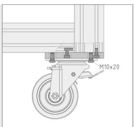
The Castor Adapter Plates for the Castor Line D125 heavy duty have the necessary through-holes in the modular dimensions of Line 8 and 12 Profiles. They also have four fastening threads M10 for castor back-plates in bore dimensions standardised to DIN 8458 - size 3.
