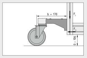
Castor Support 8 80x40 ensures that your construction has a low centre of gravity.
