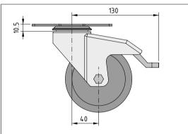
A version of item Castors D100 swivel are supplied with integrated connecting plates. As a result, the swivel castors can be secured in place without the need for additional base plates or transport plates. The three holes in the modular dimension of 40 mm in the connecting plate are used to screw the castors to the profile grooves or the core bore of Profiles 8
