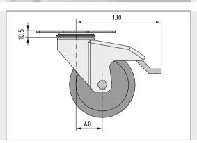
This version of Castor D125 swivel incorporates a connecting plate as standard. These swivel castors can be secured in place without the need for additional base plates or transport plates. The three holes in the modular dimension of 40 mm make it easy to screw the castors to the core bore of Profiles 8 or various profile grooves (particularly recommended for frames built using Line 8 and 10 profiles).
