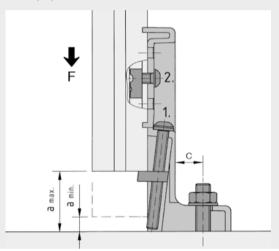
The height adjustment mechanism in the L-Based Foot enables users to compensate for unevenness in the floor. The foot is adjusted by turning the set screw (1.). The selected height is then fixed by tightening the fastening screw at the side (2.).
