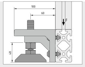
The maximum permissible load on the Foot Mounting Bracket is  $F=4,000\,\text{N}$ . The load-carrying capacity of the adjustable foot must not be exceeded.
