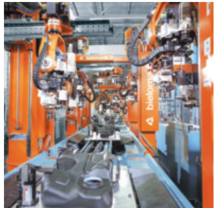
Easy Triflex® E-Chains® for multi-dimensional movements on a production line
