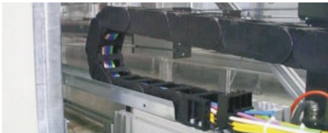
Series E4/00 with igus® Chainflex strain relief
