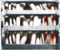
Corkscrewing: an effect of improper cable and hose placement in an E-Chain®
