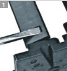
1 Lever crossbars with screwdriver
