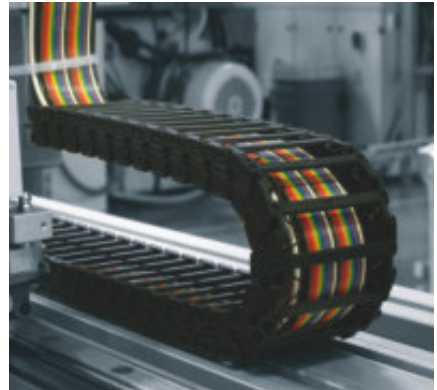
During long-term tests the System E3 with the spring band connector easily passes 15 million cycles at a bending radius of 44 mm and an acceleration of 4 g
