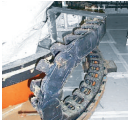
The robust link design allows also safety work in a dirty environment
