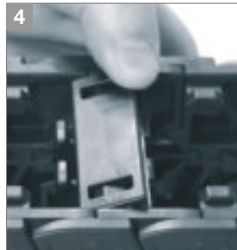
4 Position crossbars, push down and snap in
