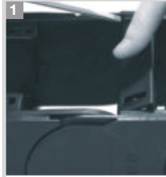
1 Remove crossbars - Insert screwdriver into the slot, push down, release by lever action
