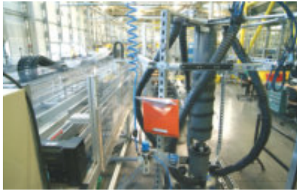
Component test - torsion tests for cables
