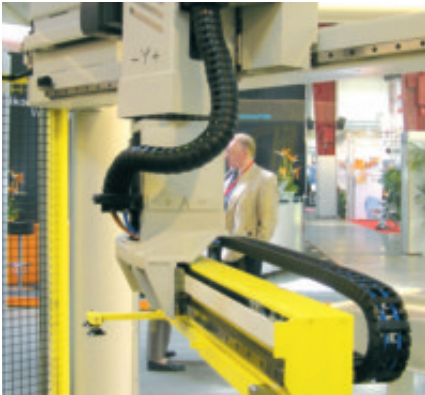
igus® System E6 and Triflex® R TRE in a Y/Z-gantry
