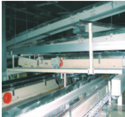
Safe energy supply also under strong dust and dirt accumulation with igus® Micro Flizz®
