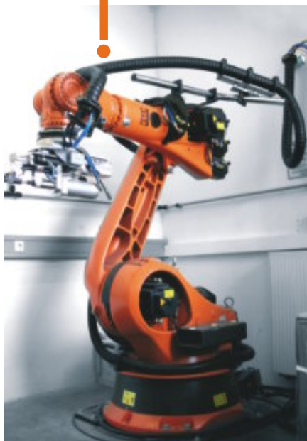
Triflex® R with fibre rods and universal assembly kit
