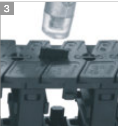
3 Gently reinsert connector by using hammer
