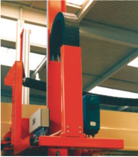
U-shaped supported E-Tube for high lateral acceleration
