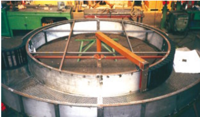
Guide troughs for rotary motion applications
