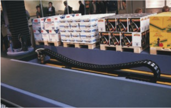
Example of unsupported permissible, FL_B
