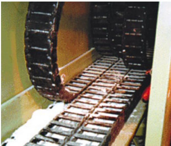
E-Chains® side by side as individual or "multiband" - Series Zipper
