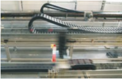
Component test - tensile strength and shear force test of igus® E-Chain®. v = 10 \text{ m/s} , a = 200 \text{ m/s}^2
