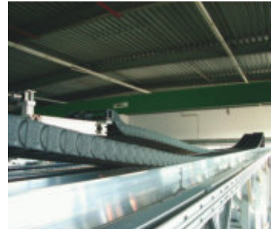
igus® Series E4/4 with super-alu-trough in a crane application
