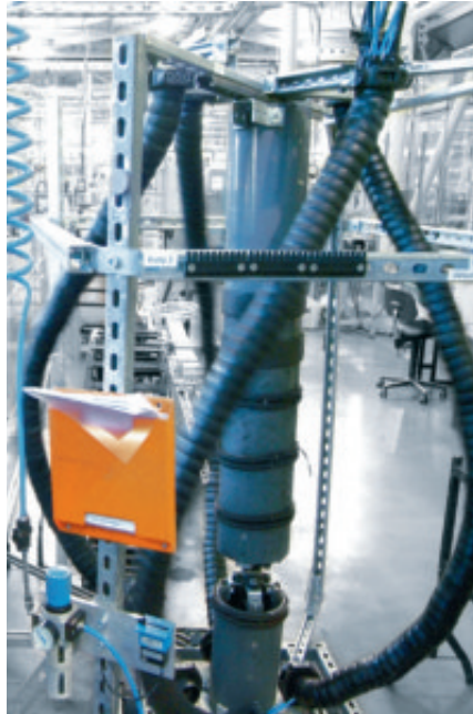
Triflex® R cable test stand with CFROBOT.037
