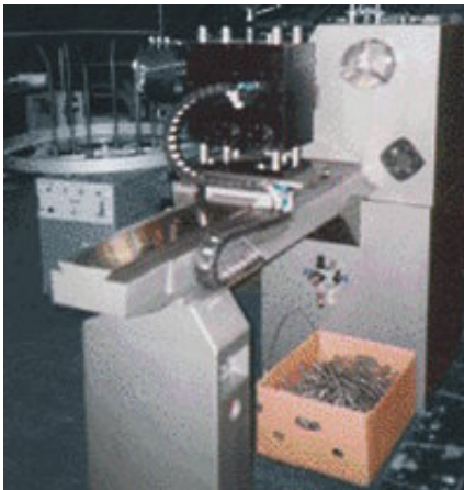
E2 mini in a milling machine with hot chips and chemicals - UL94-V2 version
