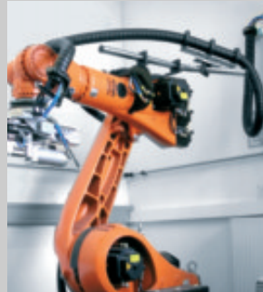
Universal assembly kit fixes fiber rod modules in any position
