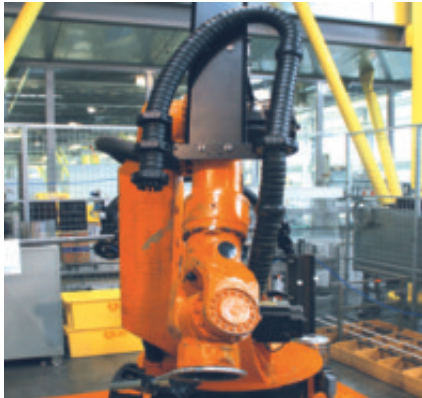
Integrated recuperating spring prevents loop formations
