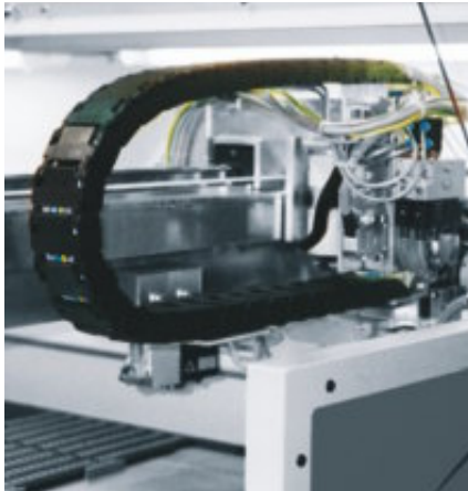
igus® E-Chain® Series 15 Zipper in automatic equipment - reduce assembly time
