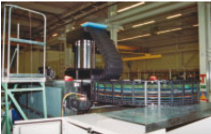
ReadyChains®, connected through a junction box, delivered by igus®, make installation even easier
