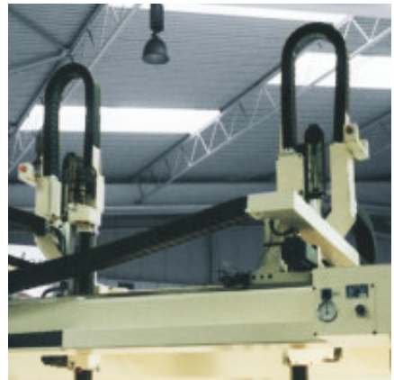
Standing application - R68 Tube - Note the first links are supported.
