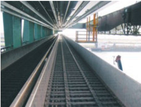
igus® System E4 with extension link at a ship loader for the coal unloading Travel 105 m, speed 240 m/min, load 53 kg/m
