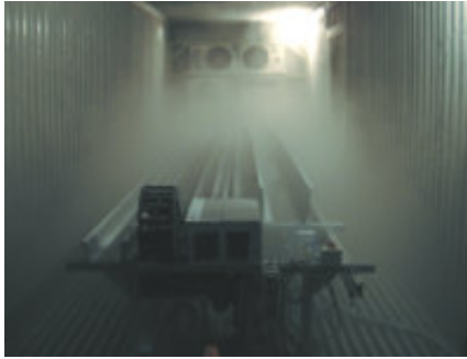
igus® climate chamber - E-Chain® and Chainflex® test runs possible at -40° to +60°C
