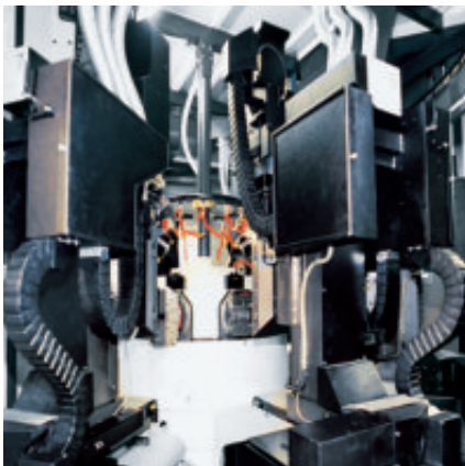
Various Triflex® tubes on the inside of a machining center
