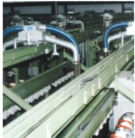
Long-travel applications up to 40 m are possible - here in textile machine
