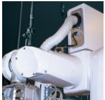
Triflex® R moulded in white color for pharmaceutical industry
