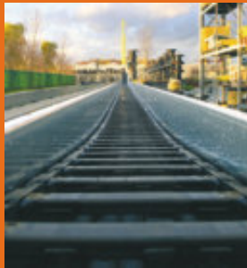
Long travel test field: 125 m travel length, speed 300 m/min
