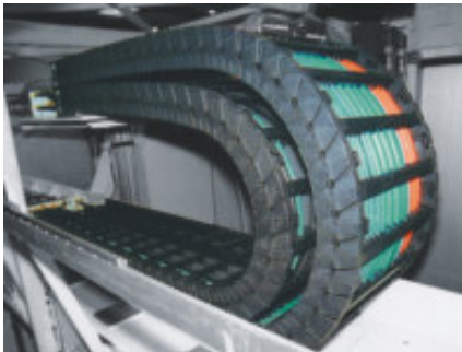
Nested E-Chains® reduce vibrations and improve milling accuracy Series E6.62
