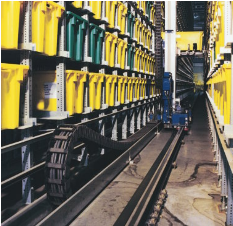
igus® steel guide trough used in a shelf conveyor application, series 350 and Chainflex® cables
