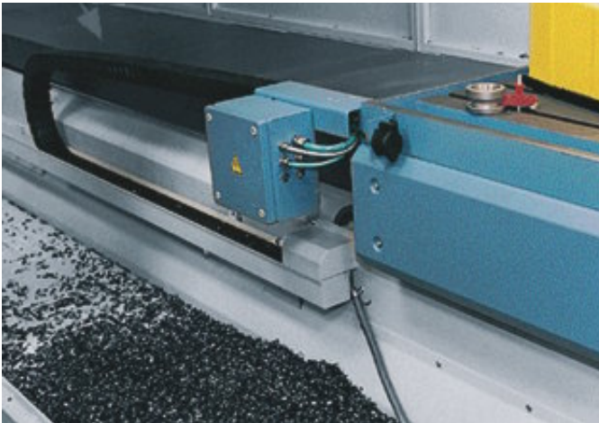
igus® E-Tubes protect your cables and are easy to open
