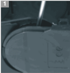
1 Remove crossbars, clips, and lids on two adjacent chain links. Guide the screwdriver into the slot between side links and release it by levering it and separate the E-Chain®
