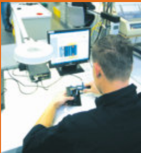
Electronic check and archiving for every chain production run
