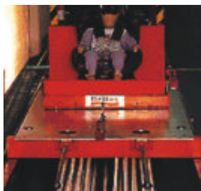
Crash test unit: 22 m/s speed and 784 m/s² acceleration, travel speed
