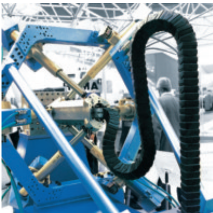
Triflex® combination of locked and flexible links to a jig
