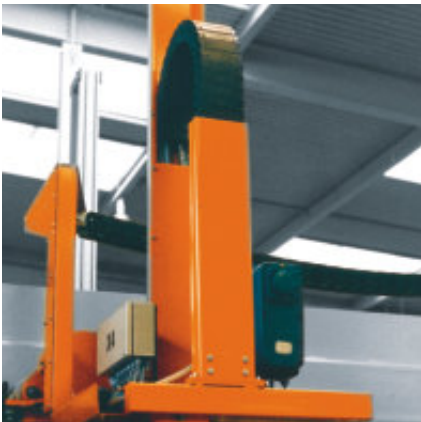
U-shaped supported E-Tube for high lateral acceleration
