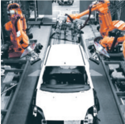
Ford, Cologne - Robots on an assembly line with igus® Easy Triflex® E-Chains®
