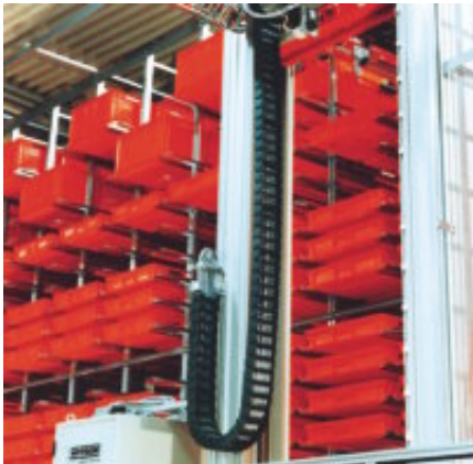
Application example: Hanging application in a high-bay storage ► page 1.20
