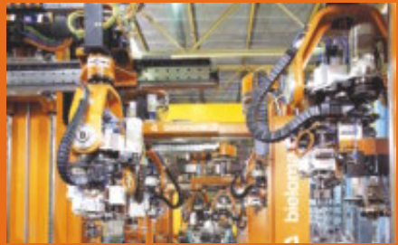
Multi-axis Easy Triflex® on a production line
