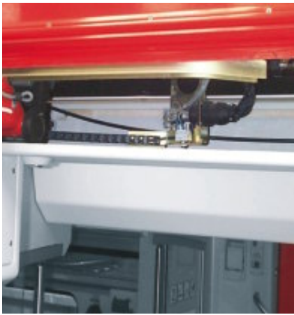
Sliding door in train - UL 94-V2 version
