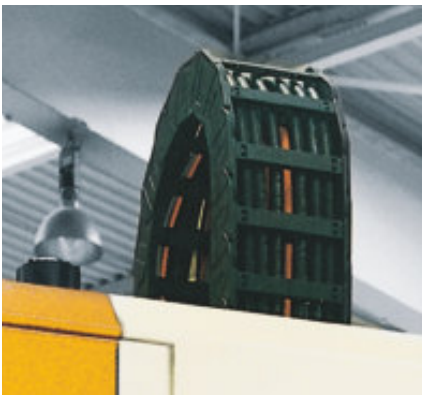
E4/light is ideal in Machine Tools with their typical short strokes
