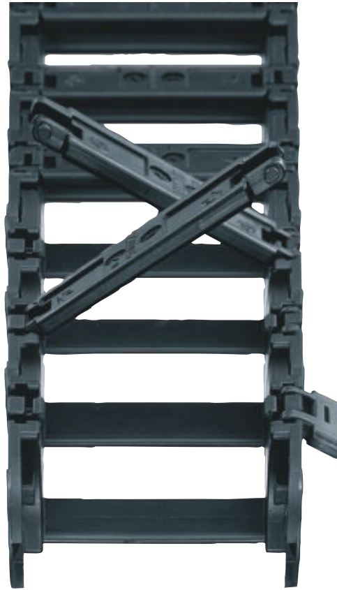
Special snap-open mechanism, choice of snap-open on left or right. Hinged crossbar can be swiveled by more than 180° on both sides
