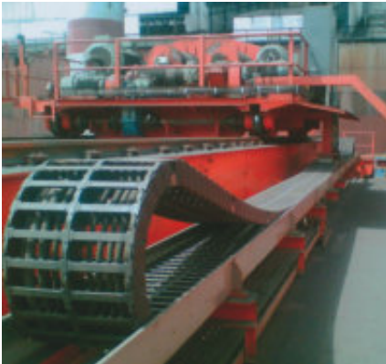
igus® Rol E-Chain® Serie 5050R in a steel plant in India with highly corrosive atmosphere - s = 22 \text{ m} , v = 1 \text{ m/s} , a = 1 \text{ m/s}^2
