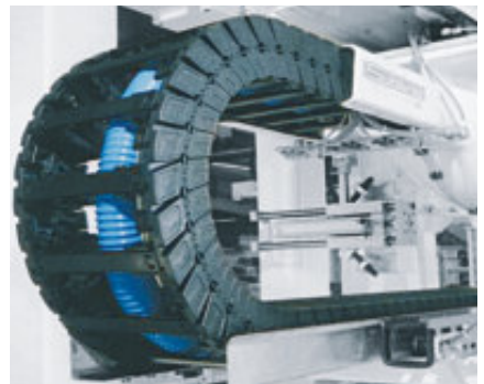
Series E6.52.150.150.0 in a pick and place robot. Handles injection molded CD covers in a split second: Tool open gripper in....tool closed - all in 0.25 seconds, speed 8m/s, acceleration: 78,5 m/s 2
