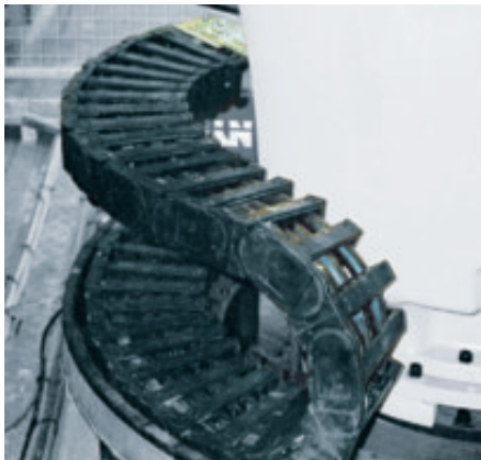
TwisterChain® for continuous industrial duty in 3-shift operation on a buckling arm robot (for welding applications, rotary movement 420°)
