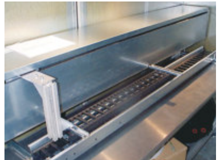
Noise test in the igus® laboratory 40db(A) E.6.29.100.100.0 series for long travel paths, v = 2 m/s
