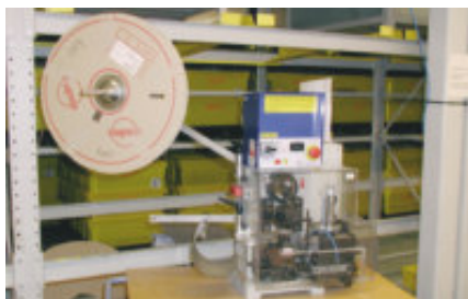
Automatic crimp machines guarantee safe connections, rationally connected
