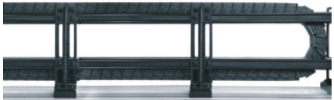
Unsupported application for very long travels. The upper and lower runs are not laid on top of each other on long travels. The lower run can also be guided "floating" without contact. Max. additional load up to 4 kg/m. Travels up to 40 m possible.
