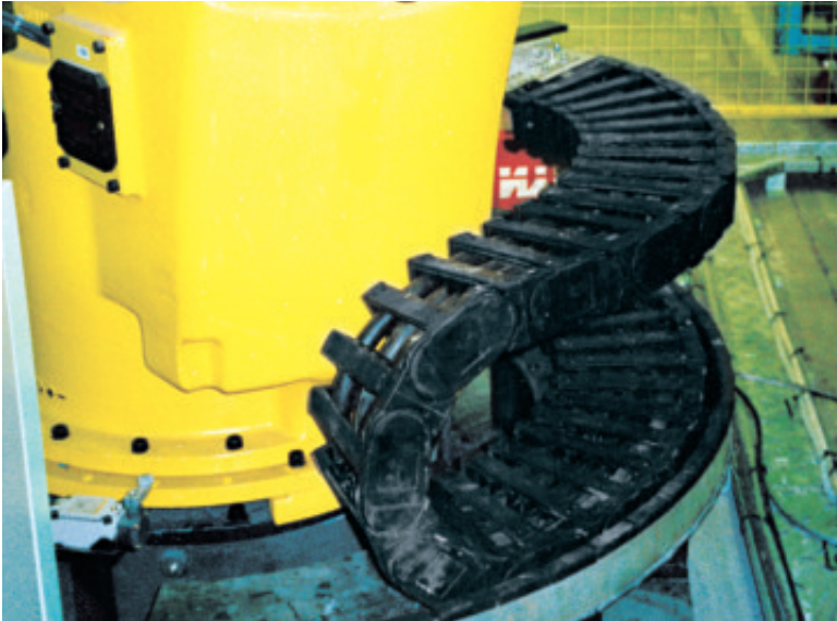
TwisterChain® for continuous industrial duty in 3-shift operation on a buckling arm robot (for welding applications, rotary movement 420°)
