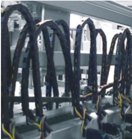
igus® E2 micro E-Chains® are robust for standing applications
