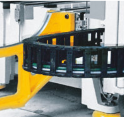
Special case: Side-mounted, unsupported - "tongue and groove" design offers stability
