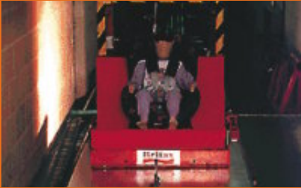
Crash test unit: 22 m/s and 784 m/s 2 acceleration for 36 m travel
