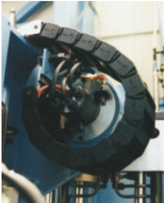
Rotary motion with a "standard" E-Chain®
