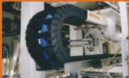
igus ® System E6 - High acceleration (8g) and ESD safety
