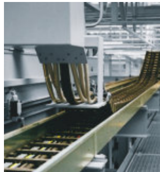
Robotics: quiet running, high acceleration, up to 10.000 cycles per day, System E4/4
