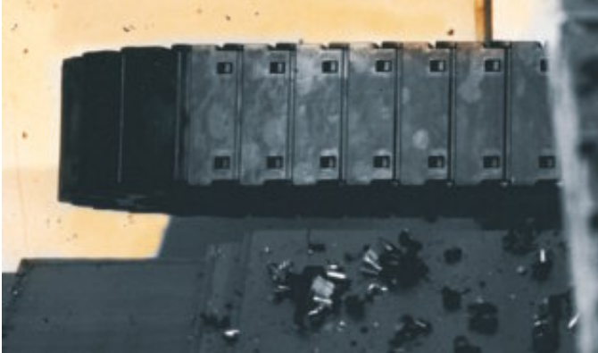
igus® E-Tubes in the chip area of machine tools
