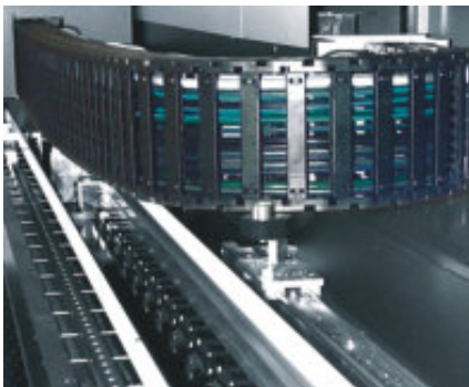
Series E6.52.050.100.0 to carry very fast electric cables and ink hoses in a digital printer, but also had to be extremely quiet and silent. Fillweight: 2 kg, v = 2 m/s, a = 20 m/s 2 , cycles per day: 6000
