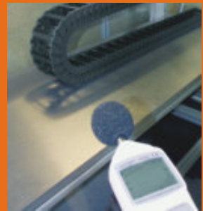
Noise level test inside an igus® acoustic cell
