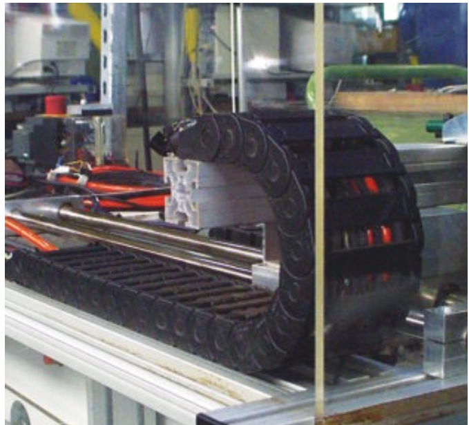
Series 255 - small pitch, smooth running - test-example at the igus® test lab
