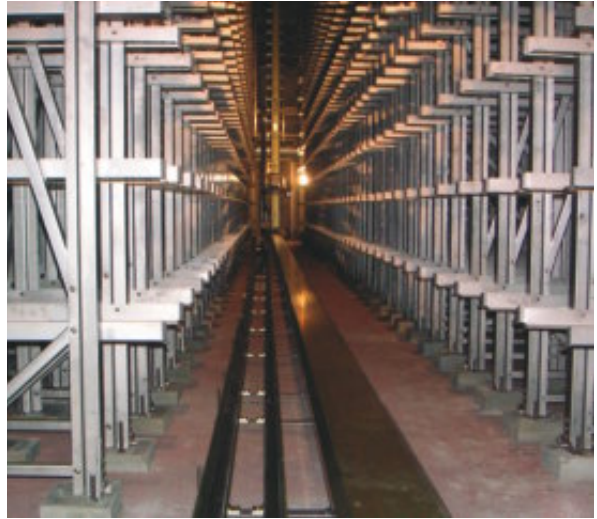
Long travel length with the super-alu-trough in a cold store
