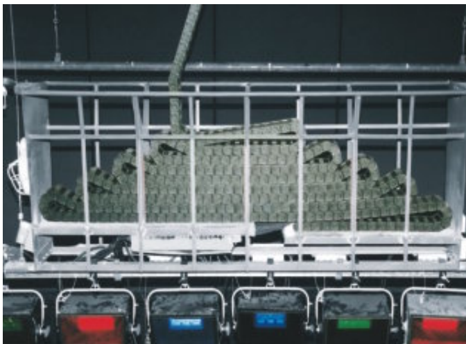
With the E-Chains® of the Systems E4 - "Zig-Zag" solutions can be realised quickly and cost-effectively without special parts
