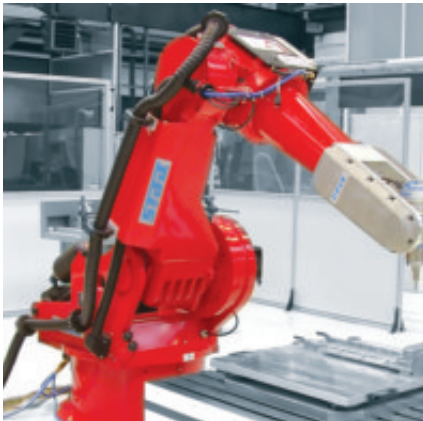
Triflex® R on a shredding robot at the Technical University of Darmstadt Source: "Advocut" project
