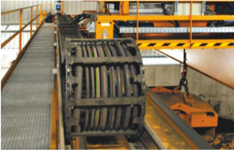
Stable guidance without oscillation. Crane operating speed 80 m/min.
