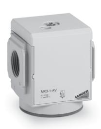
These soft start valves allow a gradual increase of the pressure in pneumatic systems. The pressure increases slowly according to the set regulation until it reaches half of the set value, then it increases rapidly. The valve poppet shifts slowly and securely to the open position to prevent sudden and unsafe movements of the pneumatic components in the system.
